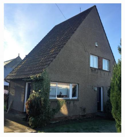
Remember, gable ends are excluded as parts of the common wall, so the common wall height for the upper portion of this dwelling is effectively zero.
