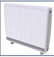
These storage heaters have advanced controls which allows a timer and often room thermostats to be used to control the system. They use smart technology to estimate heating demands based on room temperature & external temperature. They also have improved insulation.
